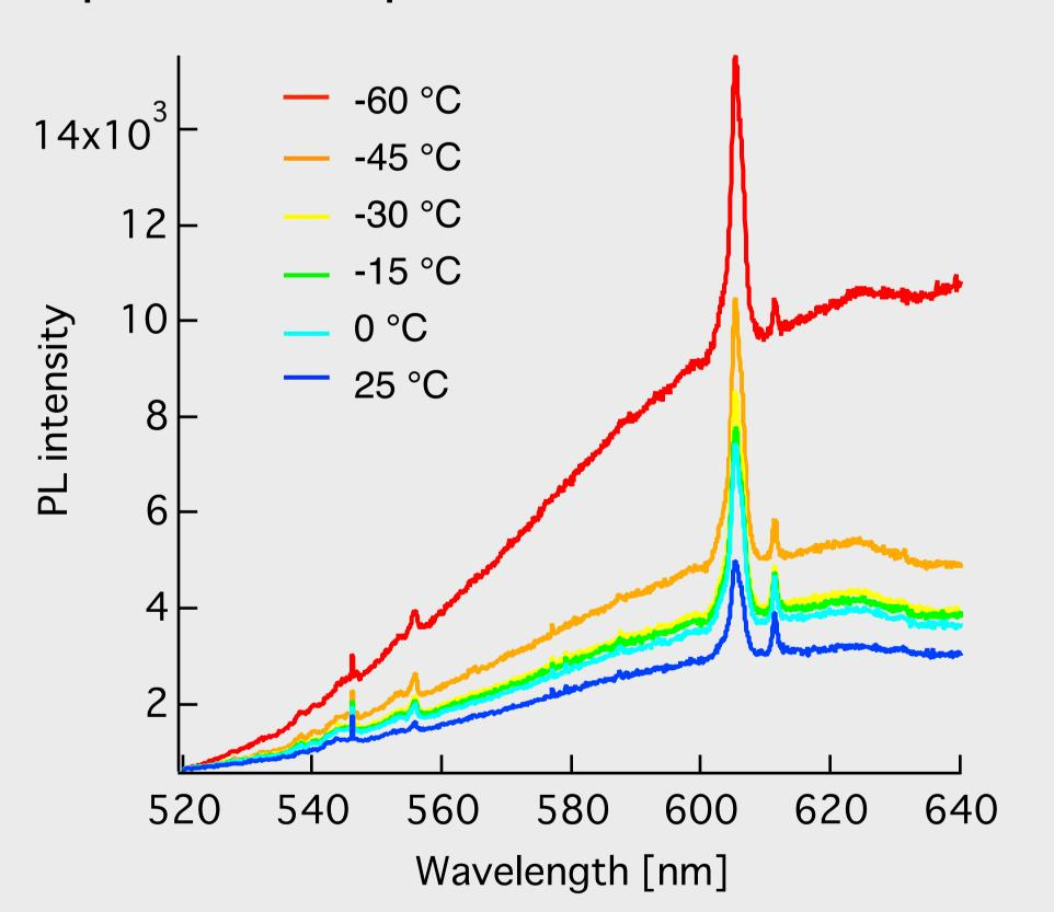
The overall PL intensity increased with decrease temperature. The enhancement originated from the suppression of thermal quenching.
