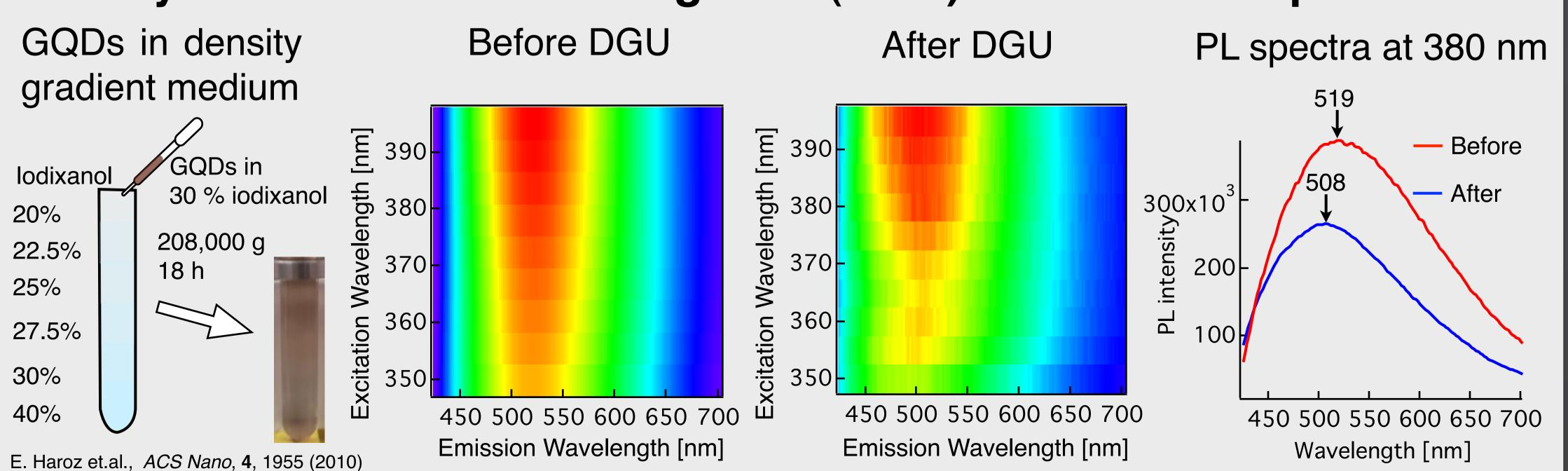
PL peaks were significantly blue-shifted by 10 nm after DGU. DGU could remove large-diameter GQDs and/or aggregated GQDs.
