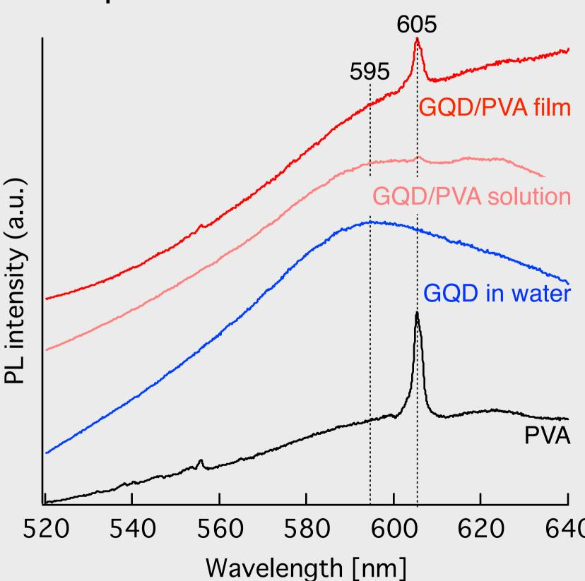
PL of the GQDs at 595 nm was suppressed when the GQDs were embedded in the film. The intensity decrease is probably related to the decrease of the concentration, the aggregation and in particular energy transfer to the polymer.
