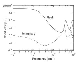
FIG. 4. Real (solid line) and imaginary (dashed line) parts of the surface conductivity of an infinitely long metallic single-wall carbon nanotube with a tube diameter of 2.7 nm, calculated according to Ref. 8.
