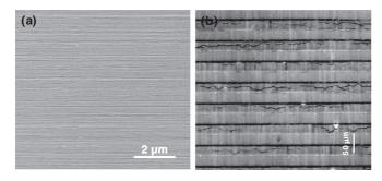
FIG. 1. (a) Scanning electron microscope image of a SWCNT film on a sapphire substrate showing the high degree of nanotube alignment. (b) Optical microscope image of the SWCNT film showing the high uniformity of the nanotube lengths.
