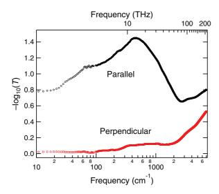
FIG. 3. (Color online) THz and infrared attenuation spectra for a highly aligned SWCNT film for polarization parallel (black) and perpendicular (red) to the nanotube alignment direction.
