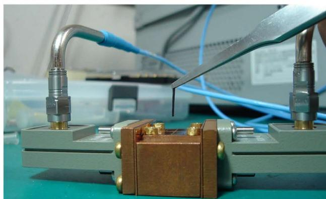
By analyzing the change in resonance, the permittivity of the nanotube sample can be calculated. Testing using nanotube samples of perpendicular orientation was used to identify the importance of orientation in the field.
