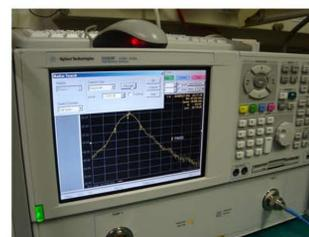
The center frequency and bandwidth of the resonance are first recorded for the empty cavity, then the signal change caused by loading a nanotube sample is measured.
