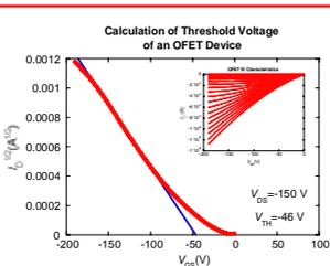
The above shows the calculation of a bipolar organic field effect transistor's threshold voltage using its I-V characteristics (inset).
