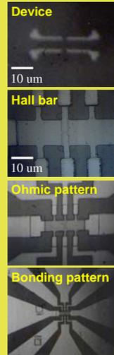
1. The ballistic rectifier device structure is exposed with electron-beam (e-beam) lithography onto the substrate and defined with wet chemical etching. The central part of the device cannot be seen in the photograph because it is too small.
