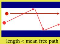
In ballistic electron transport, electrons do not collide with any impurities. Ballistic distances are only nanometers in length. Because of this, ballistic rectifiers can operate at very high frequencies.
