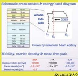
An InAs/AlGaSb heterostructure is used for fabrication as it has a very long mean free path, further increased by cooling. Buffer layers between the bottom layer (GaAs) and the channel layer (InAs) are needed to accommodate differences in lattice constants.
