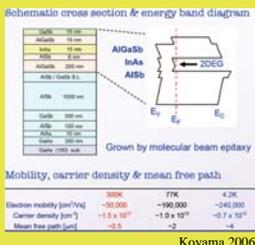
An InAs/AIGaSb heterostructure is used for fabrication as it has a very long mean free path, further increased by cooling. Buffer layers between the bottom layer (GaAs) and the channel layer (InAs) are needed to accommodate differences in lattice constants.
