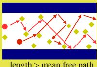
In ballistic electron transport, electrons do not collide with any impurities. Ballistic distances are only nanometers in length. Because of this, ballistic rectifiers can operate at very high frequencies.
