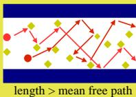
In diffusive electron transport, electrons collide with impurities in the material, scattering them and slowing them down. Traditional bridge rectifiers use diffusive transport, so they cannot operate at high frequencies.
