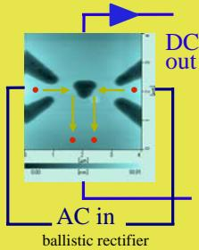
In diffusive electron transport, electrons collide with impurities in the material, scattering them and slowing them down. Traditional bridge rectifiers use diffusive transport, so they cannot operate at high frequencies.
