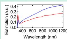
UV-vis-NIR extinction spectra of Au nanoparticles with radius of 80 nm deposited over a silver film of 20 nm thickness with a ~3 nm space layer. 2 graphs are shown because of repeatability.
