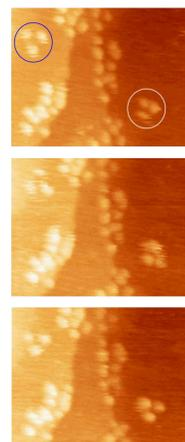
Figure 3: STM images of fullerene wheeled trimers pivoting when thermally excited.<sup>1</sup>
