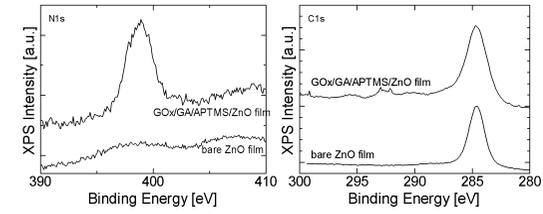
X-ray photoelectron spectroscopy (XPS) spectra of ZnO NRs/AU/Ti/Si(004) indicate that enzymes have been successfully immobilized. The XPS spectra of N1s, C1s indicates the presence of more nitrogen and carbon in treated substrates with immobilized glucose oxidase.
