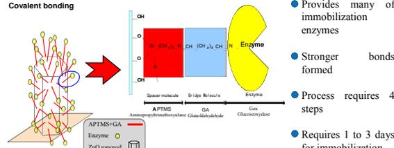
In covalent bonding ZnO NRs are treated with APTMS + toluene aqueous solution. Next the substrate is then transferred to a GA aqueous solution. To complete the covalent bonding process one drop of GOx is applied on the substrate and left for 3 days. In the case of electrostatic bonding one drop of glucose oxidase is applied on the substrate for 15 min. After immobilization a colorimetric method was used to check enzyme activity.
