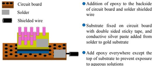
Biosensor fabrication steps stated are to ensure the substrate is in a fixed position, has a connection for parameter analysis, and has a shield against exposure. The solder selected for this experiment was 60% tin 40% lead. Epoxy was a standard commercial hydrophobic material.
