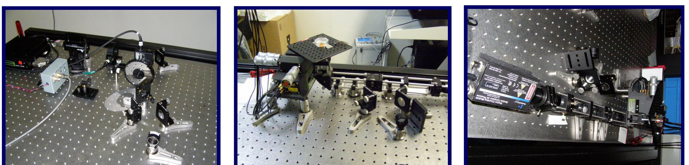
Experimental Optical Set-Up: (Left) excitation laser, shutter, ND filter, and detector to measure excitation intensity. (Middle) scanning piezo-electric stage and dichroic mirror. (Right) photon counting module collecting fluorescence from sample and objective lens.
