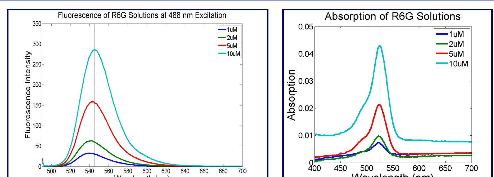
(Left) Fluorescence and (Right) absorption spectra are shown to examine the optical properties of Rhodamine 6G. The molecules are excited at 488 nm to observe the fluorescence spectra. Both spectra show a red shift with an increase in concentration. Both fluorescence intensity and absorption increase with increasing concentrations.
