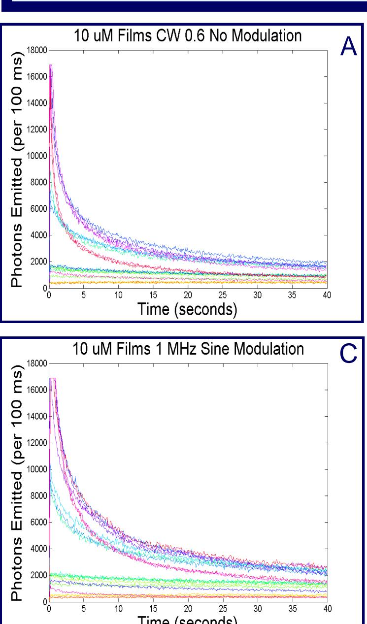
(Left) Fluorescence vs. time graphs for 4 modulation conditions. (A) CW no modulation. (B) 0.3 MHz sine modulation. (C) 1 MHz sine modulation. (D) 10 MHz sine modulation. Comparing (A) and (C) shows that sine modulation at 1 MHz gives a slower decay rate when compared to no modulation case. Comparing (B), (C), and (D) shows the effect of frequency. The optimum frequency still needs to be determined.
