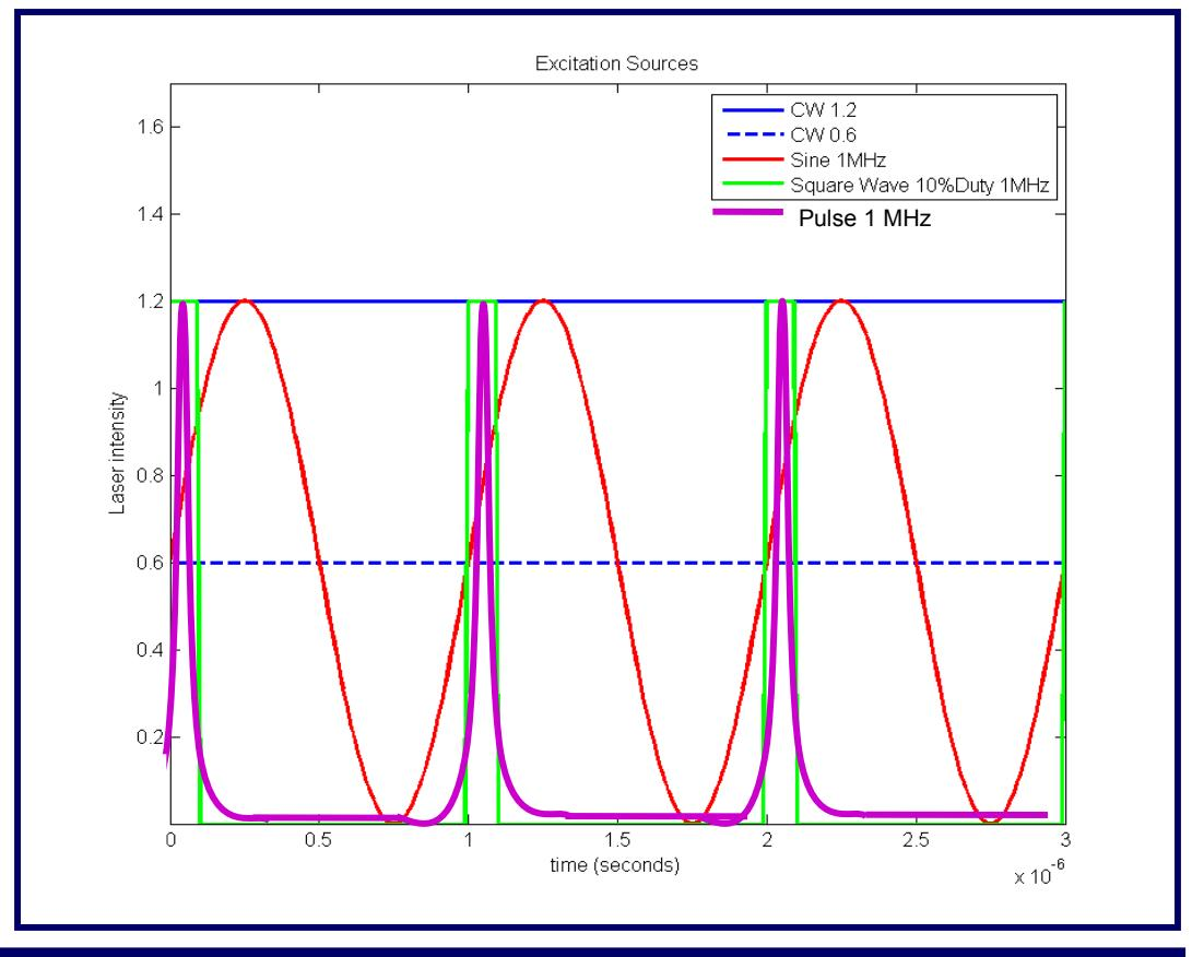
(Right) Sine, square, and pulse waves with a frequency of 1 MHz are shown. These are compared to two levels of continuous wave (CW) with no modulation. CW 1.2 has the same peak intensity and CW 0.6 has the same average power as the 1 MHz sine wave.
