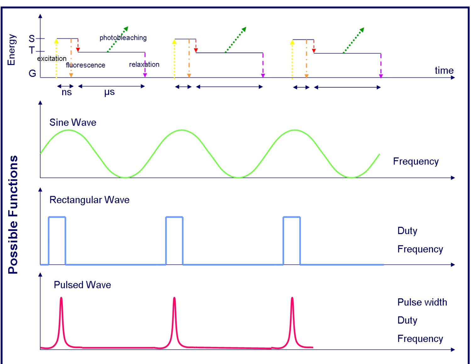
(Left) Modulation patterns line up with excitation and relaxation cycles to only excite molecules from the ground state. Possible modulation functions are shown along with parameters that can be varied.
