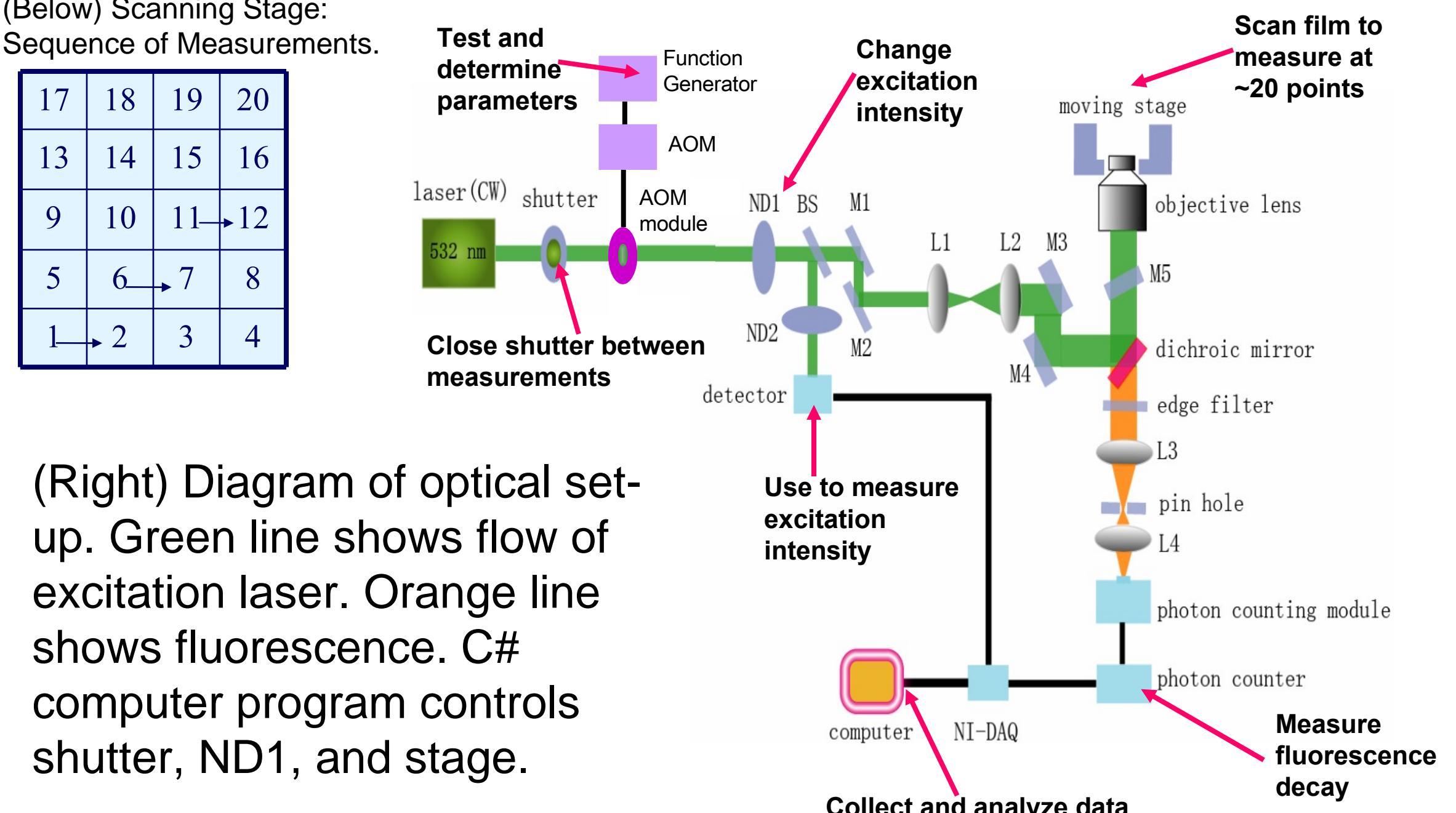
(Right) Diagram of optical set-up. Green line shows flow of excitation laser. Orange line shows fluorescence. C# computer program controls shutter, ND1, and stage.
