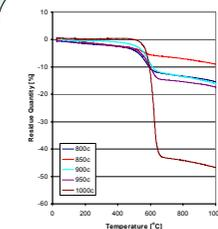
\*Since MWCNTs oxidized around 560°C and DWCNTs oxidized before MWCNTs, the higher the percentage the greater concentration of smaller tubes as well as SWCNTs and DWCNTs.
