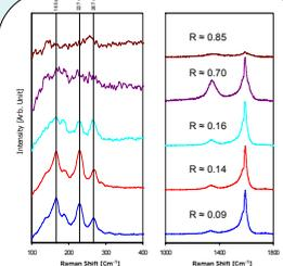
\*R value is a way to define the quality of CNTs and is defined by equation  $R = \text{Peak of D-Band} / \text{Peak of G-Band}$ . The greater the R value the lower the quality of CNTs.
